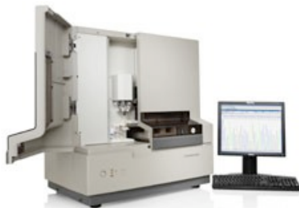
One of the capillary electrophoresis device equipped for the analysis of DNA fragments
